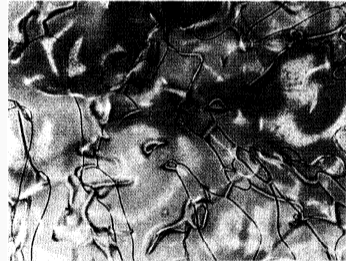
Optical microscope photograph of liquid crystal after temperature quench. [Credit: Chuang et al. 1991].
