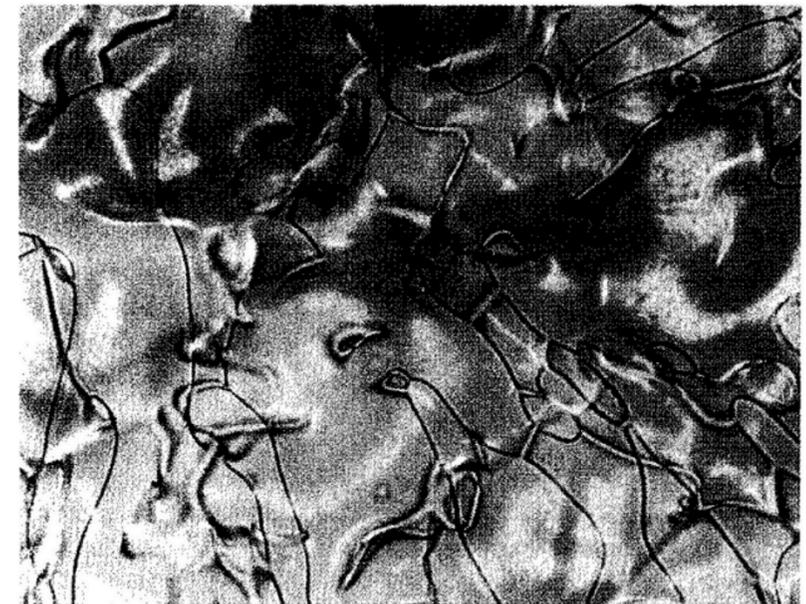
Optical microscope photograph of liquid crystal following temperature quench
